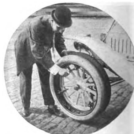
Fig. 3—Final operation, tightening nuts at ends of steel arms
